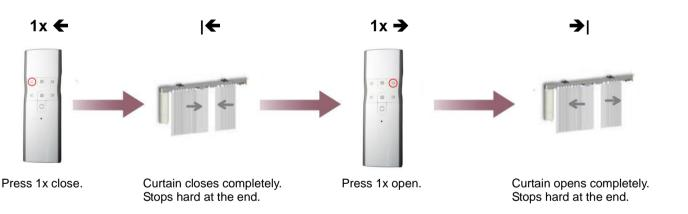
If the end positions are set with a hard stop, the curtain will stop 1 cm before the end in the future. To remove / change the end position go to Option C.
