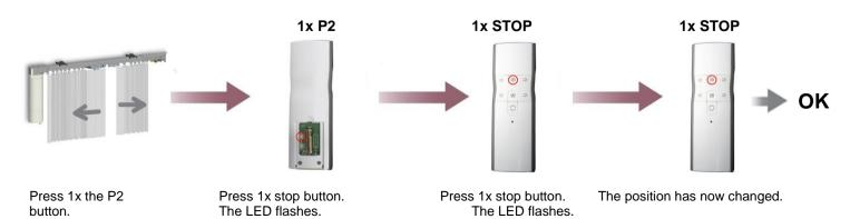
In order to remove / change the preset position, the same procedure must be repeated at the position of the preset position.
