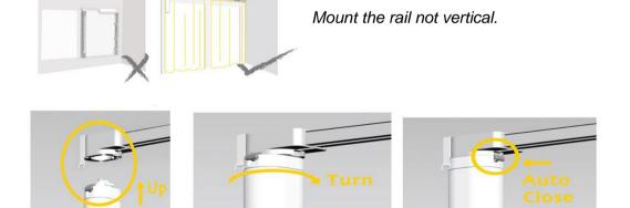
If the motor don't want to click easily, turn the gear wheel a bit and try again.
