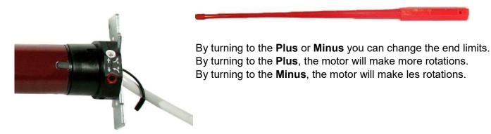
The setting needs to be done for both directions of rotation. If the motor is stopped by it selves, do not make more than one rotation to the **Minus**. This can disrupt the adjustment.
