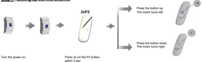
If you have made the wrong choice in the above, you can again follow the described procedure. You should turn of the power more than 3 seconds. to enter the programming mode. The above procedure also makes the memory empty, all the old programming will be removed.
