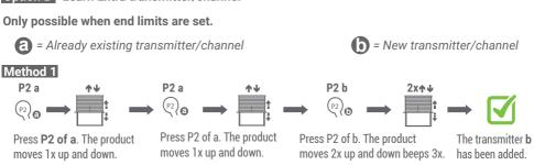
Make sure the new transmitter is in the desired channel.
