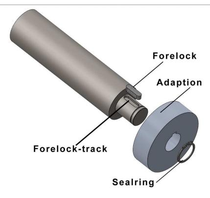
Put the forelock in the forelock-track, slide the adaptation over and fix the sealring in the dedicated slot.
