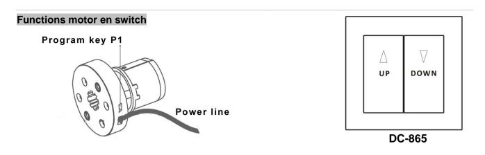
Adjusting the electronic end positions If the direction of rotation is not correct, swap black and brown cable.
